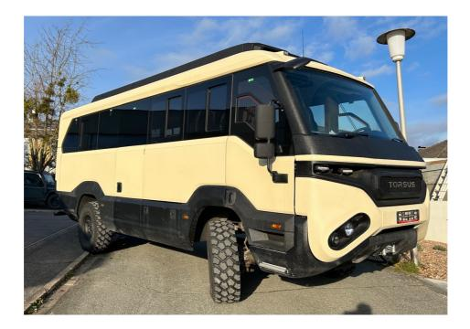
To build a proper motorhome, you need to raise the interior height of the Praetorian. For this reason, we at **ALL4BUS** have **developed a highroof.** This can be retrofitted to any Praetorian.
